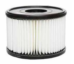
A P1 dust filter is a pre-filter that can capture coarse dust particles to protect the following filters. A P1 filter can prevent the P3 dust filter from leaking or clogging the activated carbonfilter. So the filter has an important function in a complete filter package. This filter has an F5 class and is manufactured and supplied according to the ISO16890 standard.
