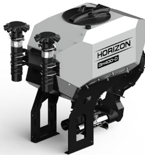
Equipped with a turbine and distribution heads to serve as a standalone seeding hopper for high outlet machines (14-64).
