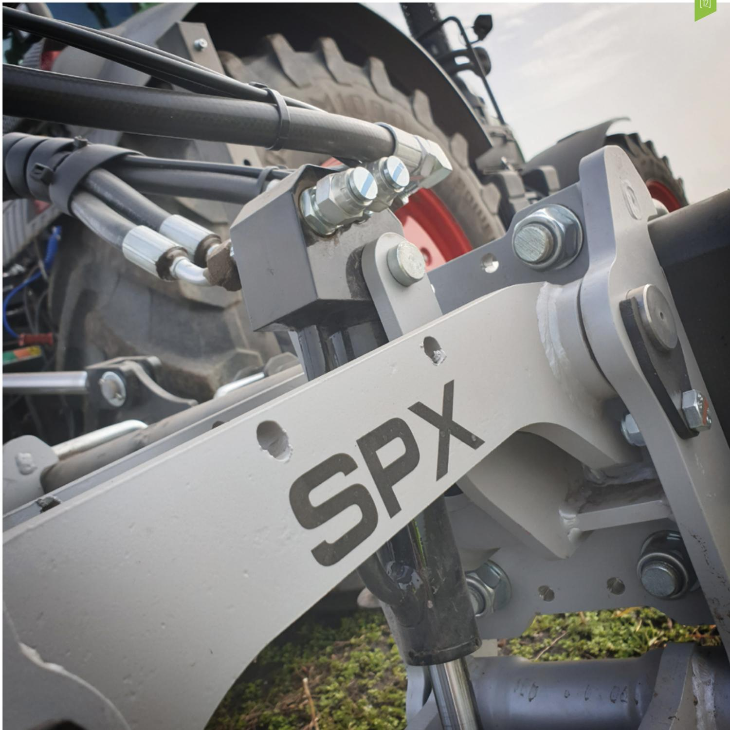
LEG WITH PIN DEPTH ADJUSTMENT
